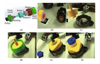
Figure 7: An example AR assembly process of an alternator [Wang et al. 2016, p. 14].
